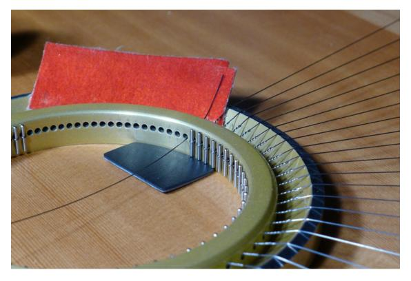
Tools and parts for stringing. The black Delrin stick is used to vertically align the hitch pins.
