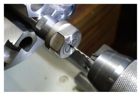
8. Mount a  $\frac{1}{2}$  in.  $\times$   $\frac{1}{16}$  in. stainless steel pin in the drill chuck and press fit it into the marker.
