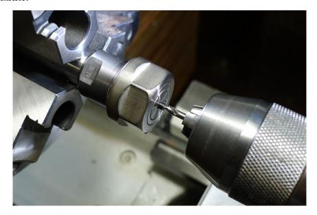
7. Drill a  $^{1\!\!/}\!\!4\text{-in.-deep}$  hole with a 0.059 in. drill bit.
