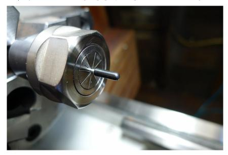
10. To seat the marker in a Delrin nut, drill a shallow flat-bottom hole with a  $\frac{1}{8}$  in. brad-point drill bit.
