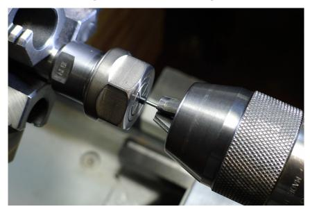
9. Mount the stainless steel pin in a collet chuck and round over the top end of the marker with a fine file. Sand the marker with wet/dry 600- and 1000-grit paper, and polish with a buffing wheel.
