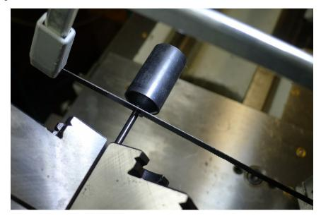
4. Mount the marker in a collet chuck and face it on both ends.
