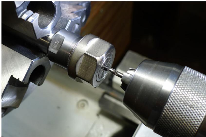
7. Drill a  $\frac{1}{4}$ -in.-deep hole with a 0.059 in. drill bit.
