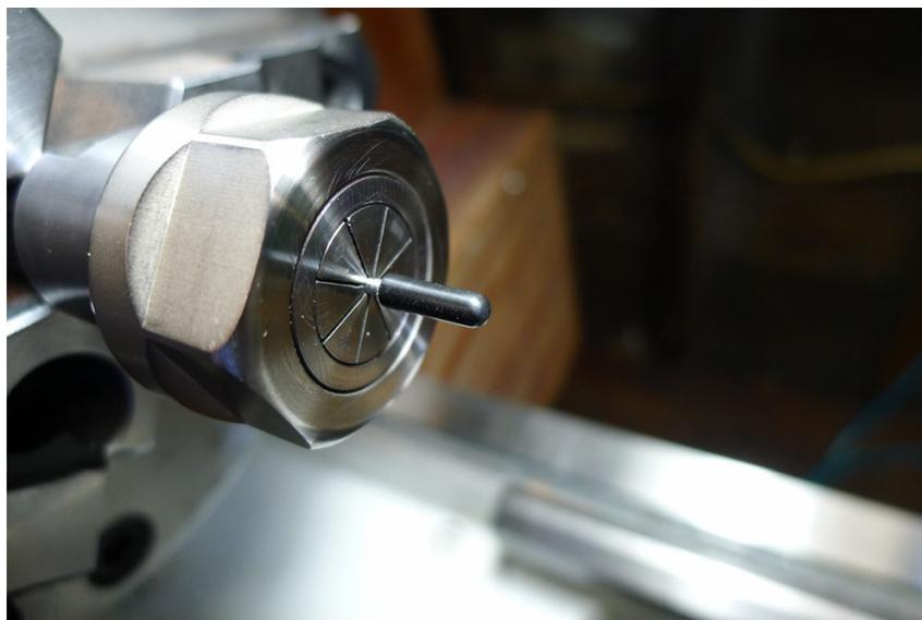
10. To seat the marker in a Delrin nut, drill a shallow flat-bottom hole with a 1/8 in. brad-point drill bit.
