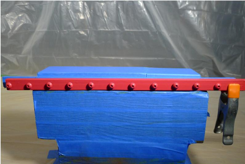
With the buttons in a horizontal position and the stick handle on the right, spray the second pass.
