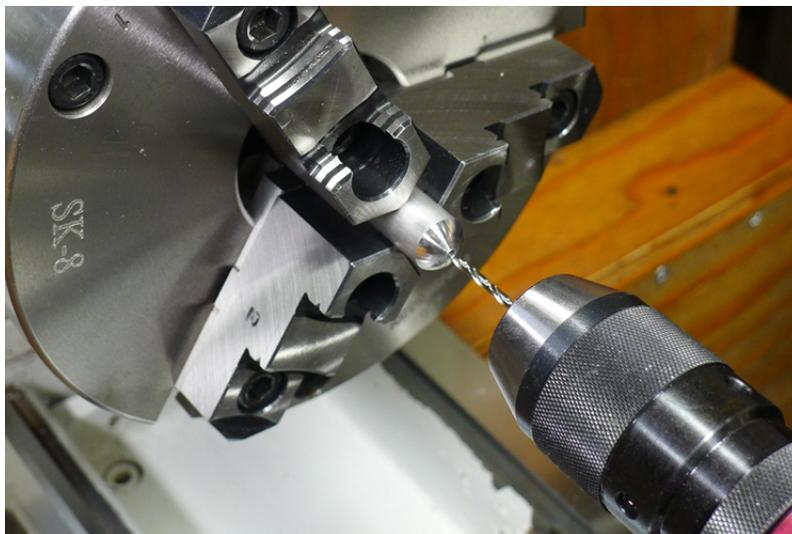
7. Set up a carriage stop to ensure that all holes have the same depth.
