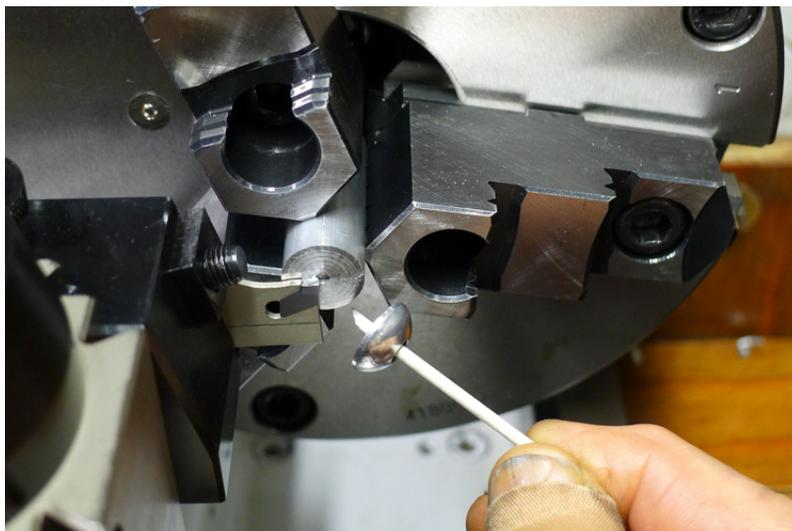
10. Mount the buttons on a custom-made mandrel with a 4-40 tapped hole in the center. Fasten the mandrel in a drill chuck secured in the lathe chuck. Set up a  $\frac{1}{16}$  in. concave radius tool bit at approximately  $45^\circ$  to the bottom edges of the buttons. Lock the carriage and round over the edges. Finished button diameter: 0.605 in.
