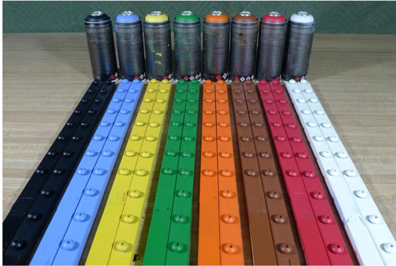
17. The cans of the *Montana Black* line of paints come with orange-tipped nozzles that produce a round-shaped spray pattern. In contrast, all the cans of the three Montana primers mentioned above come with yellow-tipped nozzles that produce either a vertical or horizontal fan-shaped spray pattern.
