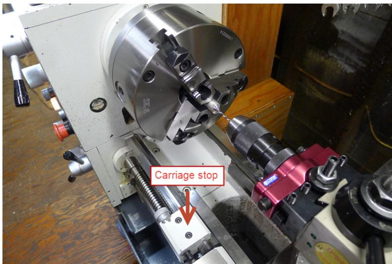
8. With a #4 counterbore — Weldon LGN4-1 — drill holes 0.130 in. deep.
