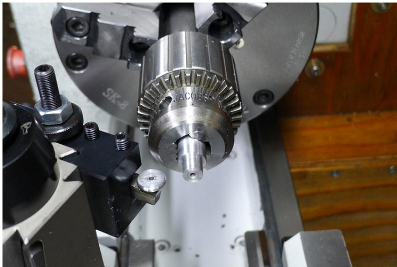
11. Drill out the centers of all  $\frac{1}{4}$ -20 soundboard machine screws and thread them with a 4-40 tap. Fasten the buttons to the machine screws with 4-40 socket head cap screws. Chrysalis I screw length:  $\frac{3}{8}$  in. Chrysalis II screw length:  $\frac{1}{2}$  in.
