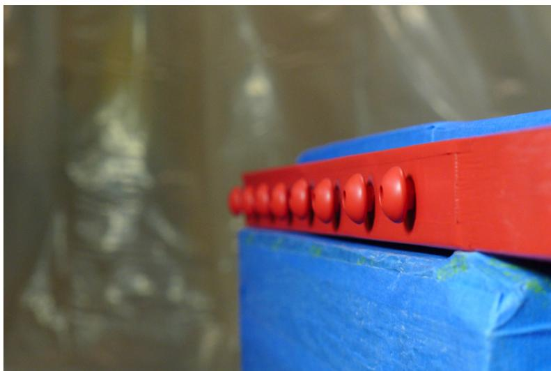
16. Each coat of primer and paint consists of three passes. With the buttons in a vertical position and the stick handle clamped on the right, spray the first pass. *Remember, do not hold the cans at an angle.*
