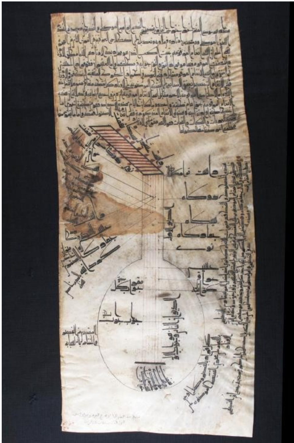
Drawing of an oud from al-Fārābī's (d.950) manuscript of Kitāb al-mūsīqā al-kabir : It appears to have seven strings and fourteen mālāwī , which means the use of double strings.
